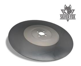
**SILVER FOX**, P.V.D multi-layer coating with a thickness of 2.5 microns, opaque grey colored. The particular composition and the innovative mix of noble elements developed by our R&D achieves a hardness which is higher than 3.650 Vickers (HV 0.05), unattained by any other coating. It's suggested for cutting high alloy steels up to 1000 N/mm², stainless steel and all material developing high thermal energy.
